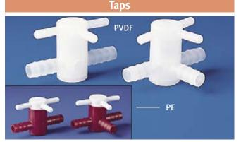
Taps with 2 or 3 channels, Polyethylene has excellent chemical resistance, The PDVF is autoclavable and can withstand temperatures up to  $+204^{\circ}$ C, Maximum pressure : 34.3 kPa (5 psi),
