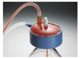
For high-speed sterilisation of 5 to 10 litres by vacuum filtration.
